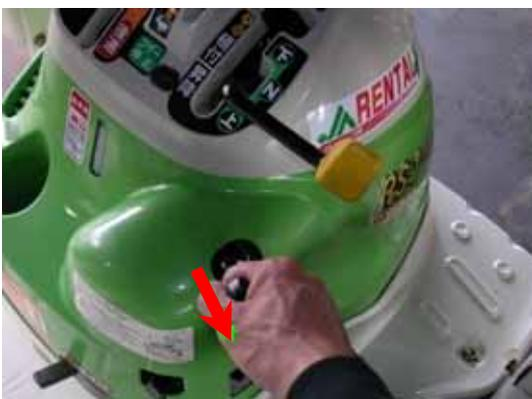
A photograph showing a person's hand pulling a yellow-handled starter lever on the engine control panel. A red arrow points to the lever. The panel also features a "RENTAL" sticker and other controls.                                             |
