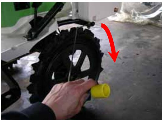
A photograph showing the front marker being pulled out from the machine. A red arrow indicates the outward direction of removal.                                     |
