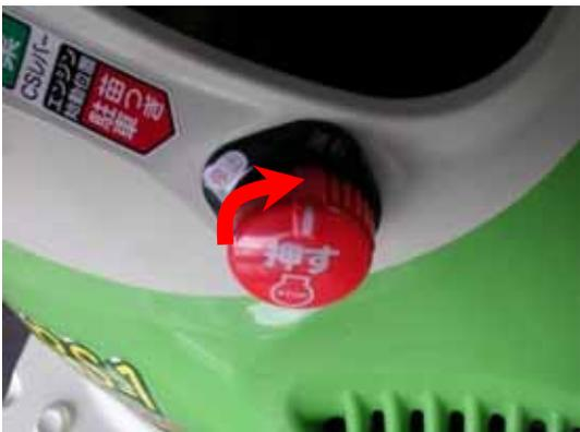
A close-up photograph of the red stop button. A red arrow is drawn on the image, pointing clockwise from the top of the button, indicating the direction to rotate it.                                                                                |
