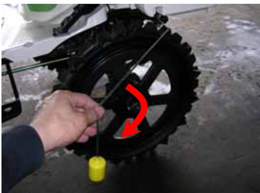
A photograph showing the front marker being turned downwards. A red arrow indicates the downward direction of the turn.                                              |
